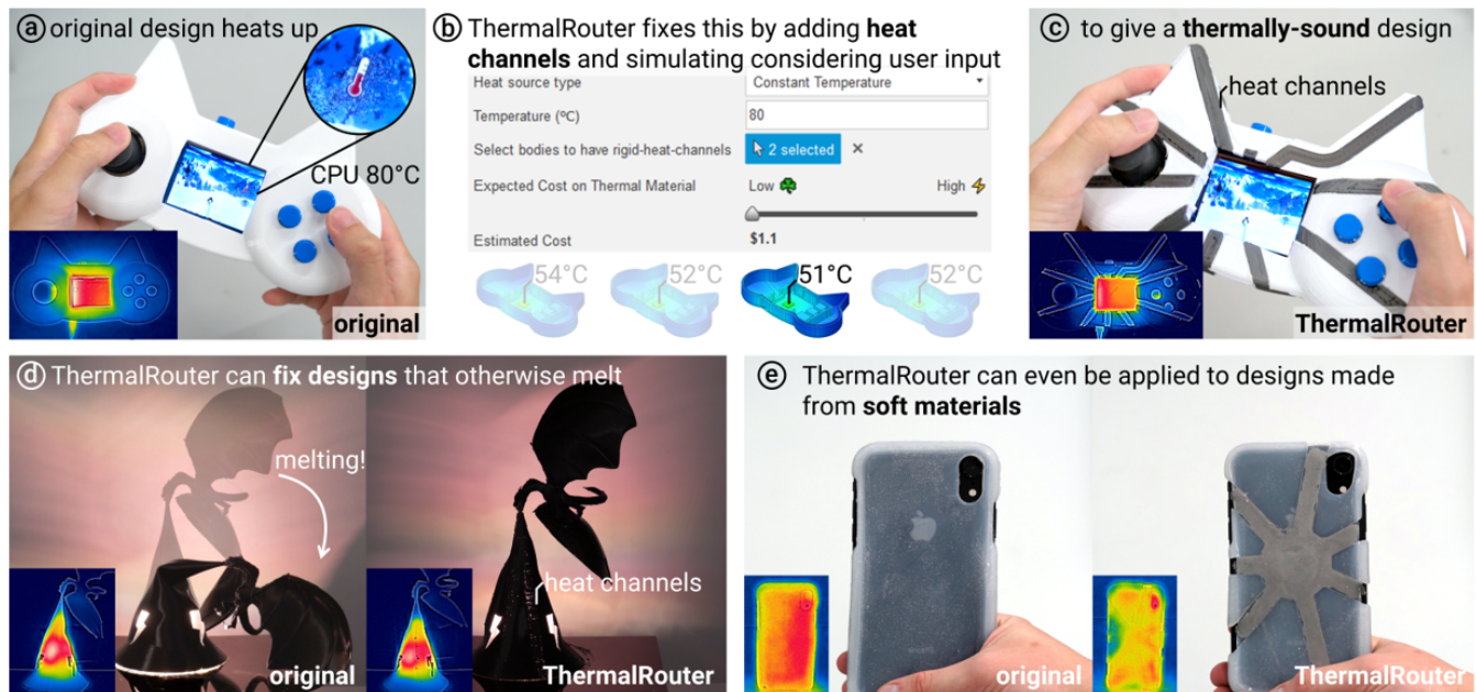
Figure 1: Three objects improved using ThermalRouter: (a) 3D-printed game console slowed due to CPU heat. (b,c) ThermalRouter added thermally-conductive channels to route heat away from the heat source. (d) 3D printed dragon lamp melted at PLA’s heat deflection temperature; ThermalRouter created a version that didn’t buckle. (e) ThermalRouter can also be applied to soft objects like a silicone phone case with embedded liquid metal channels.
