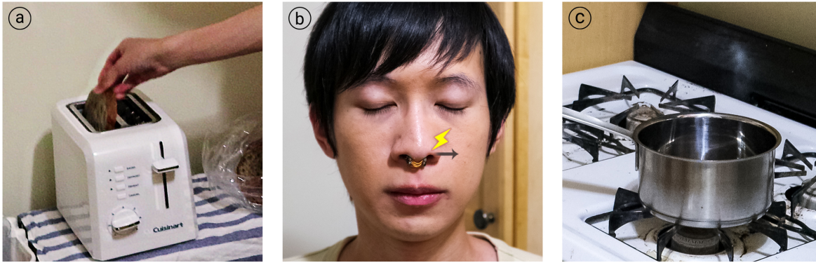
Figure 2: (a) Our user burnt their toast while making breakfast, which unfortunately emits a strong odor that masks the actual danger, a gas leak in their stove. (b) As the user inhales, our device renders the smell of methane by stimulating the user’s trigeminal nerve electrically and to the left—indicating the location of the methane gas leak, which is tracked via an external odor sensor that relays these readings to our sensor via Bluetooth. (c) This allowed the user to find the leak.
