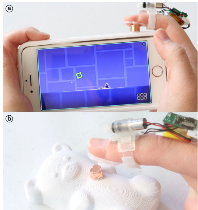
Figure 12: Examples of altering softness of regions on fully rigid 3D printed objects (made from PLA).
