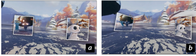
Figure 5. (a) Without the tilt, flat 2D PIPs degrade the immersive experience. (b) With the tilt, 3D PIPs can blend into a 3D environment.
