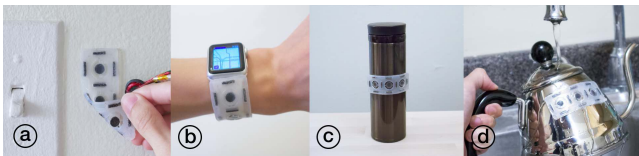
Figure 6: (a) The user peels off the patch. Because our interactive patches are passive and soft , they can be applied to a variety of objects: (b) smartwatch bracelet, (c) water bottle, (d) and even washed (still works while wet).
