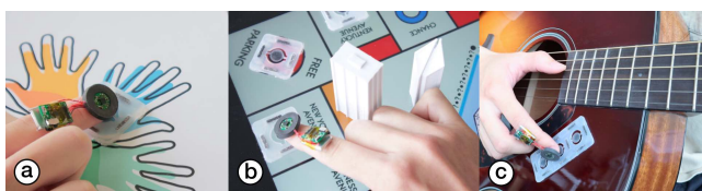
Figure 22: Examples of how MagnetIO can enhance everyday objects by creating an ad-hoc I/O space; these objects can now sense touch interactions and vibrate in response.
