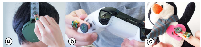
Figure 23: Examples of how MagnetIO patches can conform to objects of various shapes.
