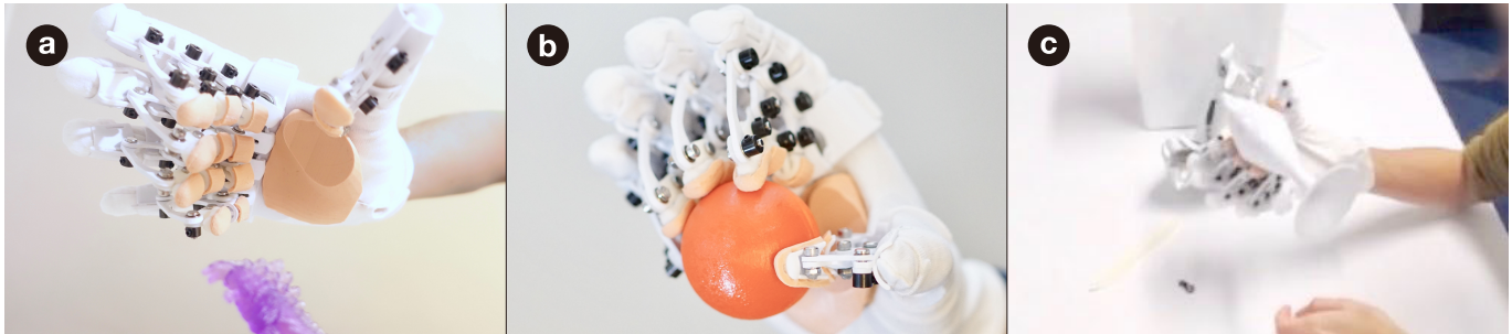
Figure 1. (a) We engineered a passive exoskeleton, HandMorph, that approximates the experience of a smaller grasping range. HandMorph uses mechanical links to transmit motion and haptic feedback from the wearer’s fingers to a smaller hand. (b) In our first user study, we found that participants perceived objects as larger when wearing HandMorph, which suggests that their size perception was transformed. (c) HandMorph achieves this transformation in the user’s real environment. As such, it can, for instance, allow a product designer to change their grasp into that of a child while evaluating a toy. In fact, our second study found that participants felt more confident in their toy designs when using HandMorph to validate ergonomics.
