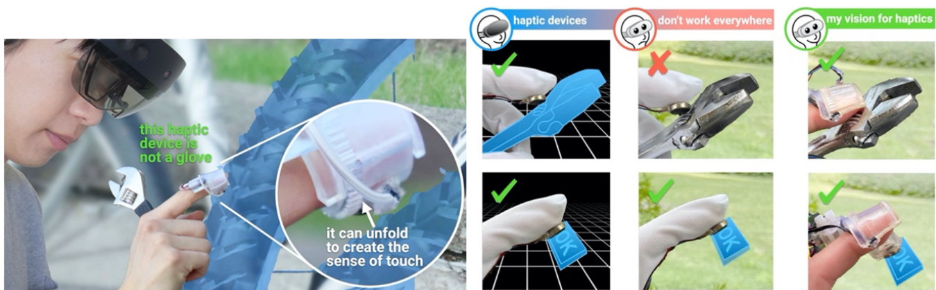
Figure 2: (left) My finger-worn haptic actuator (Touch&Fold) allows the user to feel the sense of touch from virtual object, yet the device folds back after the interaction, to allow the user to feel physical objects. (right) Unlike many haptic devices that work only for VR, my vision is to engineer devices that works in all realities, enabling haptics anywhere .
