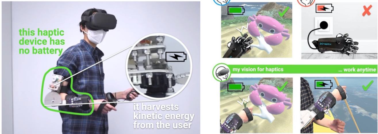
Figure 3: (left) My arm-worn haptic device has no battery, and it harvests kinetic energy from the user. (right) Unlike many haptic devices that run out of battery very soon, my vision is to harvest energy from the user, while they are enjoying multisensory interactions, enabling haptics anytime .
